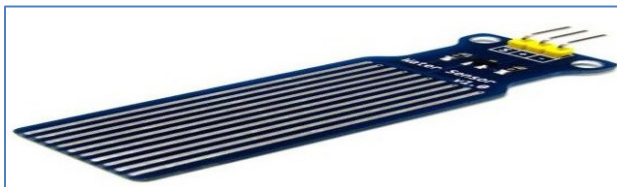
Figure 10. Physical representation of water sensor
