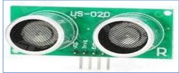
Figure 11. Physical representation of ultrasonic sensor
