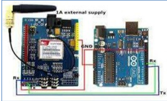
Figure 9. Connect the GSM 900 with Arduino mega
